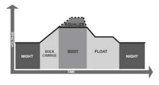
Figure 4-2 Tracer-BN series MPPT charging algorithm
