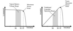
Figure 4-1 Nominal 12V Solar Module I-V curve and output power graph
